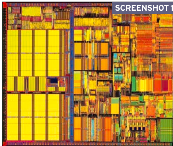
The circuit diagram of Intel's Pentium III processor, launched in 1999. Later versions running at 600MHz or higher proved particularly good for overclocking experiments, but some PC systems will prevent you from adjusting bus speeds
